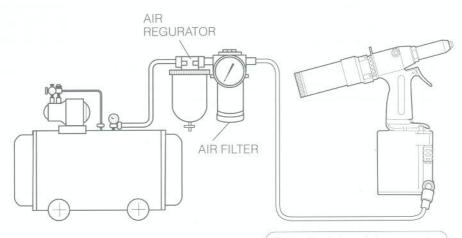
Either the left or right connector can be used. Be sure to insert the change plug into the connector which is not being used.
